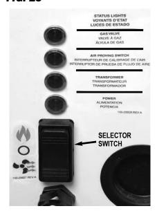
When the switch is set to heat, four status lights (see Fig.15) will be activated in sequence as specific circuits are checked by the ignition control. If the heater does not light, and a status light is off, refer to the troubleshooting label on the inside of the heater's burner end access door or the troubelshooting of the manual.
